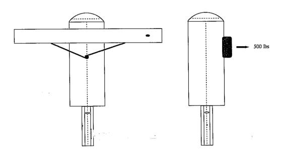
Test #3- Shear test on bolt holes
